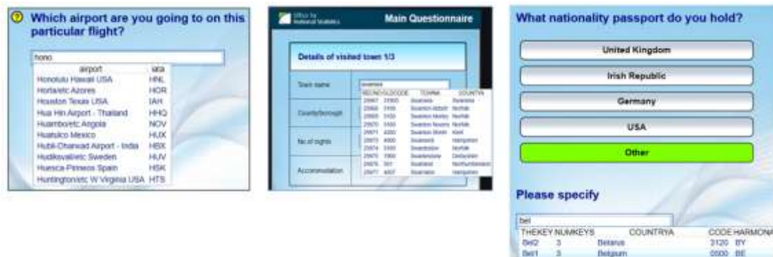
Figure 7 - Lookup text box with Trigram search is the most suitable implementation for fields where the user may be unsure of the correct spelling e.g. airport codes, UK towns, country codes
